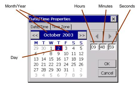
You can change the month and year using the two buttons stated (<< and >>). You can select the day directly by touching the day of the month. Hours, minutes and seconds are changed after they are selected with the buttons shown above. Hours must be entered in 24 hour format. Touching «OK» will cause the current settings in the clock module to be saved and retained, even in the event of a restart.
